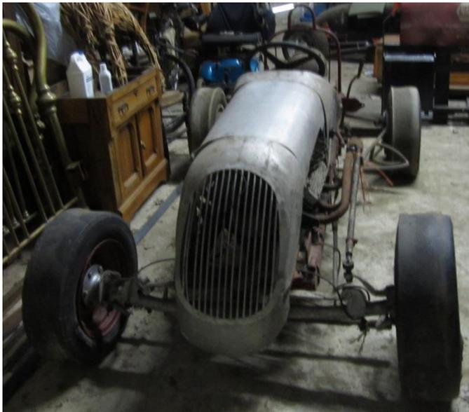
Some stats: The racer has a modified 1934 Plymouth frame, Model T front springs and suspension, a 1937 -39 Ford V8 60 horsepower engine, an Eddie Meyer dual intake carburetor. The tires were made for an asphalt track.
